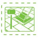
A slab and paver roller compactor or a rubber mallet can be used to compact NOCO<sup>™</sup>.
